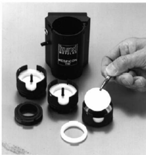
fig. 5.4.1 - 1 RESPICON and its three stepped collection system
