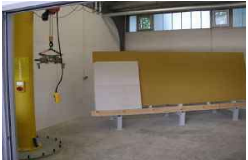
fig. 5.3 - 4 A-support for material reception in test room
