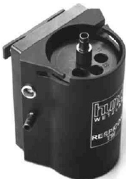
fig. 5.4.1 - 1 RESPICON and its three stepped collection system
